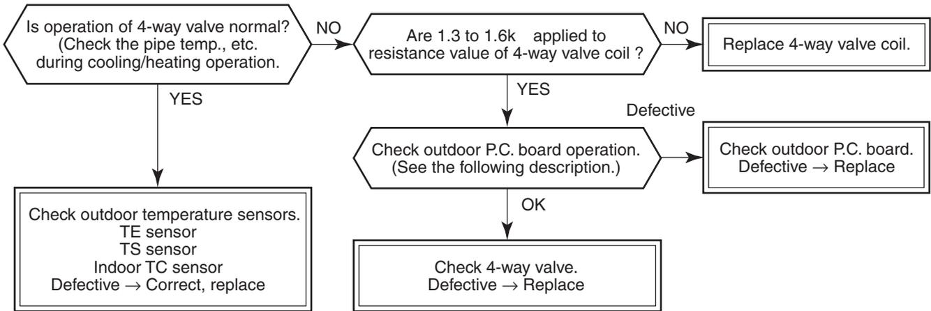
**Operation check direction of the outdoor P.C. board (In case of self-preservation valve)**
